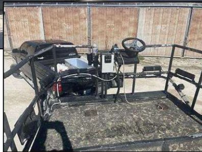
Forward Deck - Air Motor Steering
